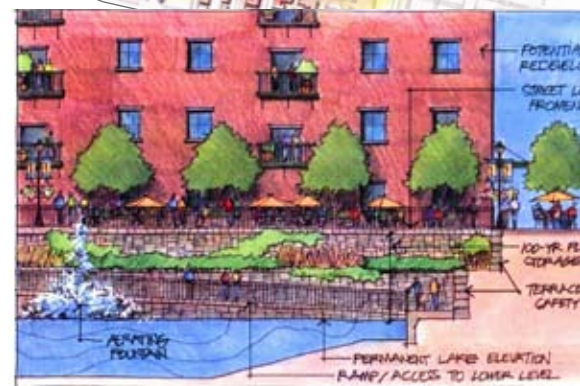
Development in Tulsa’s Pearl District may include stormwater management systems that also serve as water features.
