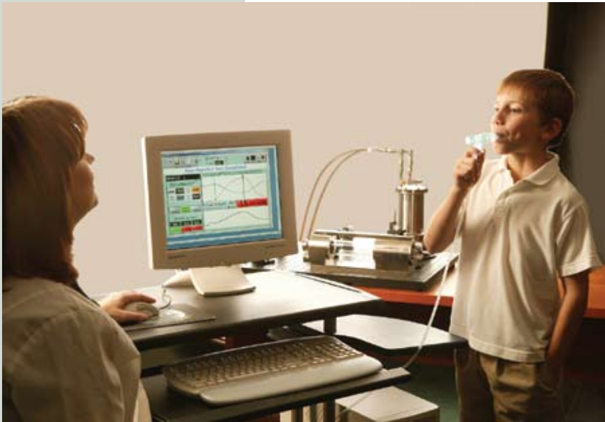
A nurse assists a child in providing a breath sample using the Breathmeter, a device that detects biomarkers for diseases/conditions like asthma, diabetes, schizophrenia and cancer.
