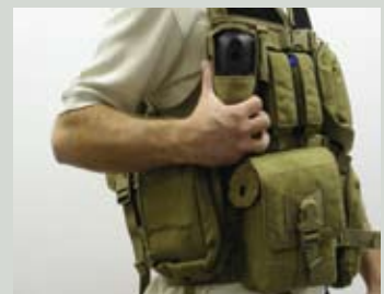
The BioBadge® portable personal air sampler is worn by an individual to monitor exposure to biological organisms.
