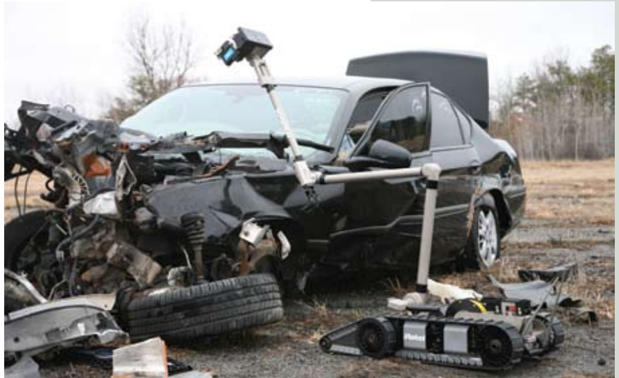
Fido® OnBoard examines vehicle wreckage for explosive devices, vapors or particulates.
