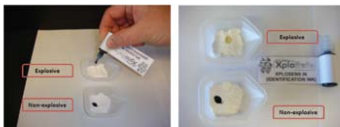
(left) Explosive identification test using XploSens Explosive Identification Ink. (right) The ink reacts with the explosive compound to turn from dark blue to yellow/tan.
